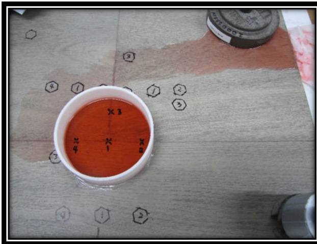
Sample 1 - Water was able to channel through the joints and puddle on the surface of the planks.
