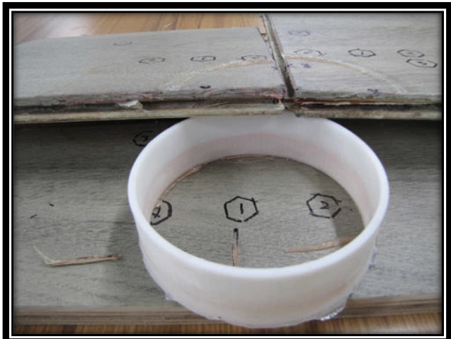
Sample 1 - Water was able to channel through the joints and puddle on the surface of the planks.
